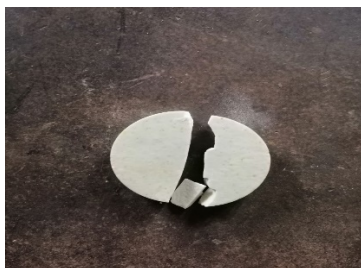
Figure 4: Fracture pellet after DTS test
